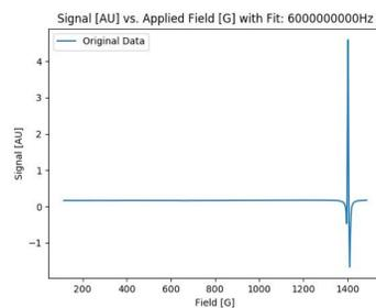
Fig 2. A plot of the output signal vs magnetic field. FMR position is seen around 1400 G at 6 GHz.
