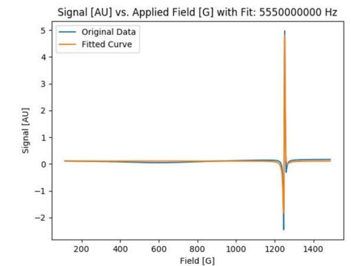
Fig 5. A fitted curve for output signal vs magnetic field at 5.55 GHz, used to find the calculated FMR position.
