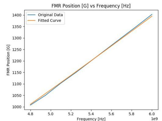
Fig 6. The fitted Kittel equation used to determine and compare computed values of the gyromagnetic ratio and sample magnetization.
